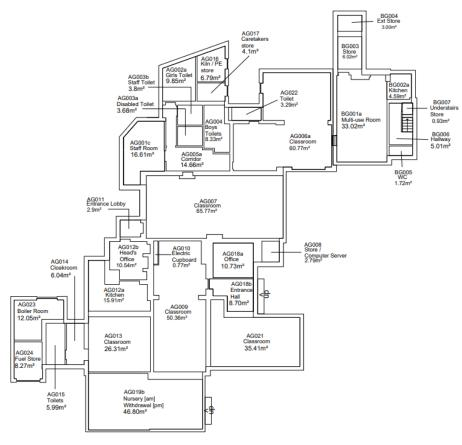
GROUND FLOOR PLAN - Block A Gross Internal Area = 487.72m<sup>2</sup> Gross External Area = 532.00m<sup>2</sup>
